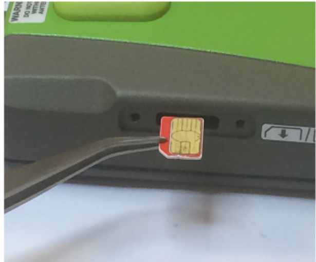
Figure 2. JLink LTE micro SIM card installation
