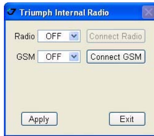
Figure 2-12. ModemVU TRIUMPH Internal Radio selection
