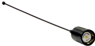
UHF NGP Antenna 406-430/430-450/ 450-470 MHz, 1/2, 2.4 dB gain, NMO p/n 99-587307-01 (optional)
