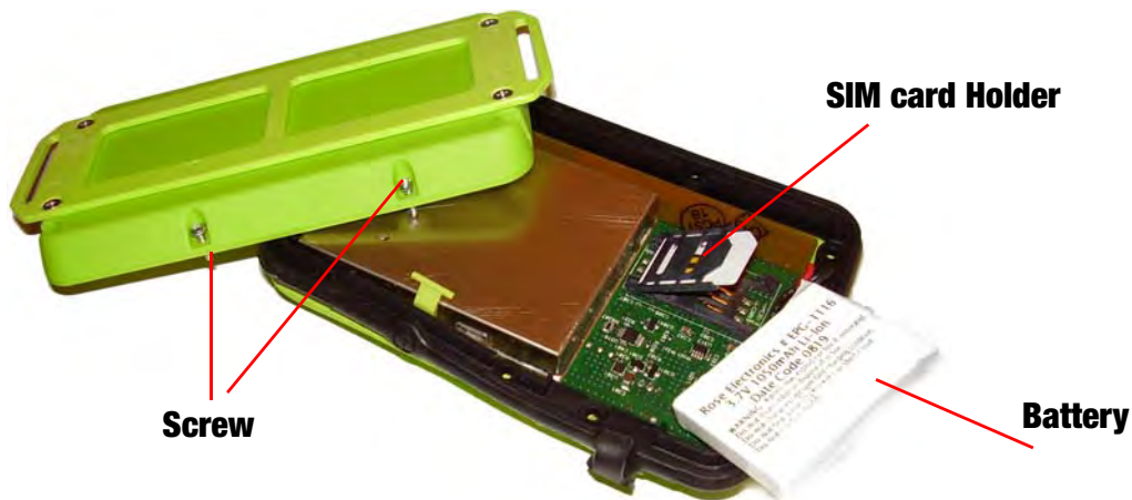
Figure 3. SIM Card installation
