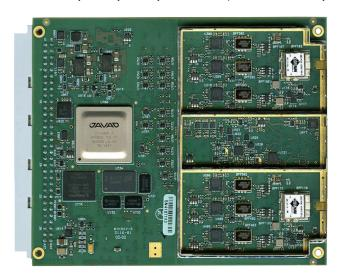
864 GNSS channels of this board allow tracking all current and future satellite signals. TRE-DUO is a board that accepts inputs from up to two antennas. It is equivalent of two receivers which operate synchronously with a common oscillator and central processor to coordinate all communications and other activities.
