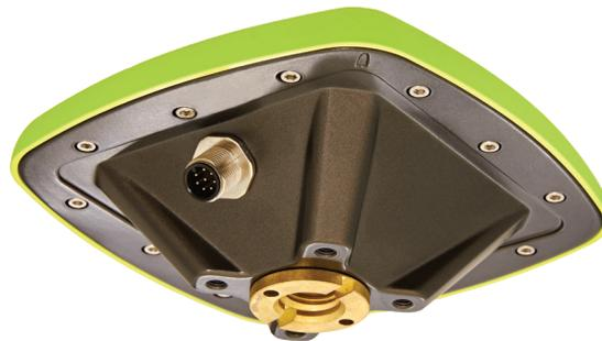
GyrAnt is a versatile, high-performance antenna (GrAnt) that combines the Inertial Measurement Unit (IMU) and the GNSS antenna. It can be mounted on flat surfaces with four screws or mounted on standard poles (5/8-11 or 1-14 inches thread).
