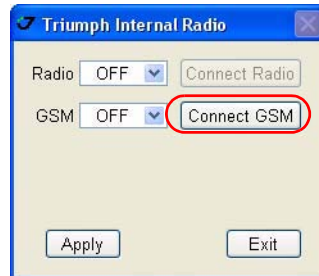
Figure 1-7. ModemVU TRIUMPH Internal Radio selection
