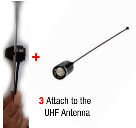
2 Place the Ground Plane between cable parts and screw all together
