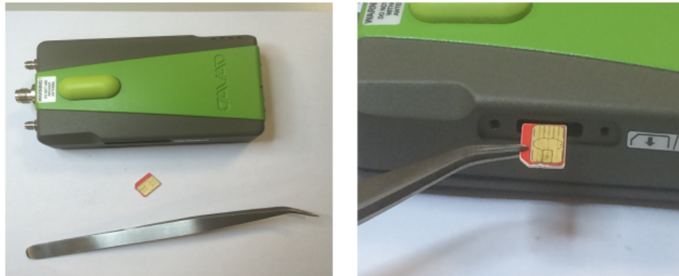
Picture 2. JLink LTE micro SIM card installation procedure
