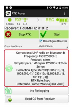
Check the UHF radio settings, and tap Apply to save Tap the Start button to start the RTK Survey. them and apply.
