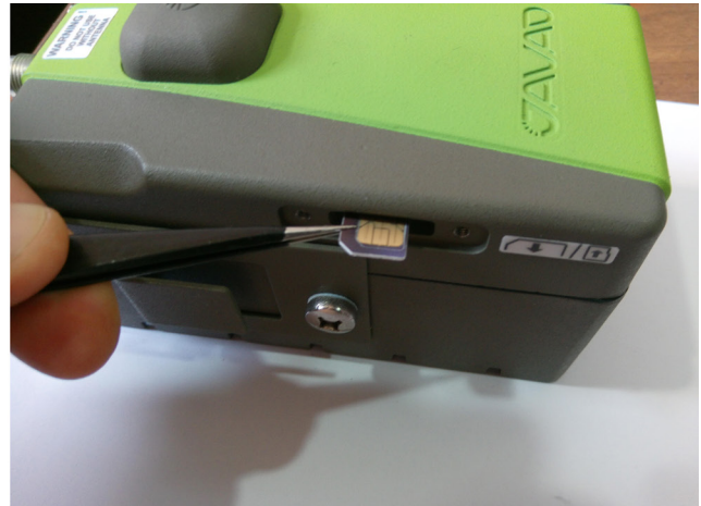
Figure 2. HPT435BT JL micro SIM card installation
