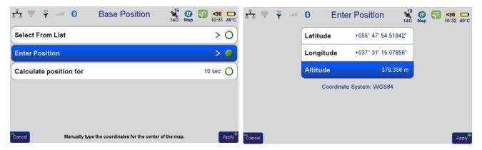
Figure 44. Base station position
