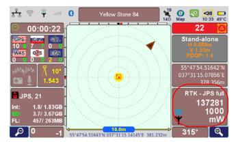
Figure 75. Base station is transmitting corrections
