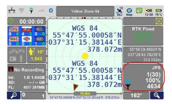
Figure 85. Rover is receiving corrections
