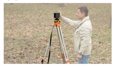
Figure 14. TRIUMPH-VS on tripod
