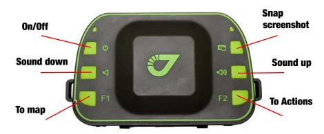
Figure 4. User programmable buttons and On/Off button
