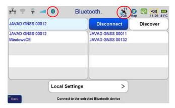
Figure 58. TRIUMPH-1 is connected to TRIUMPH-VS
