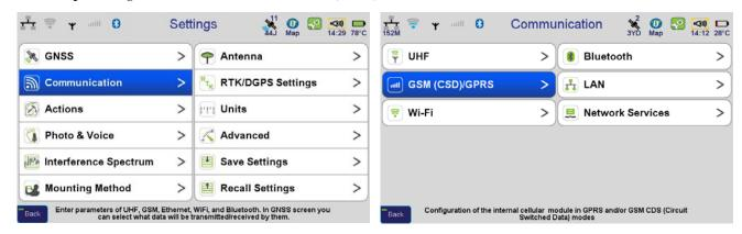
Figure 46. Communication ➤ GSM (CSD)/GPRS
